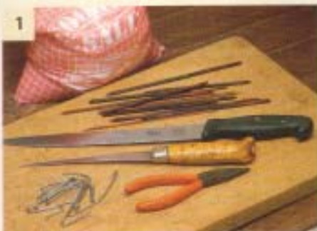
1 The tools for the job — knives, pliers, bamboo stakes and metal hooks.
